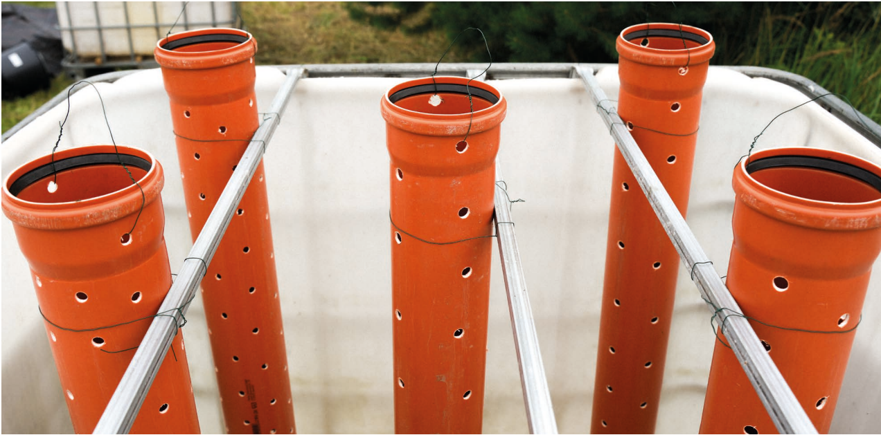
Shown here: a Johnson-Su bioreactor with five aeration pipes before filling. In 2024, eight different compost variants were created and tested to develop the optimal composition for various soils. Through targeted formulas, these variants can now be applied according to specific needs, ranging from arable farming to agroforestry.
